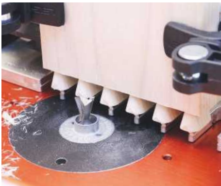
▲ Half-blind dovetails show the usual rounded profile when routed
